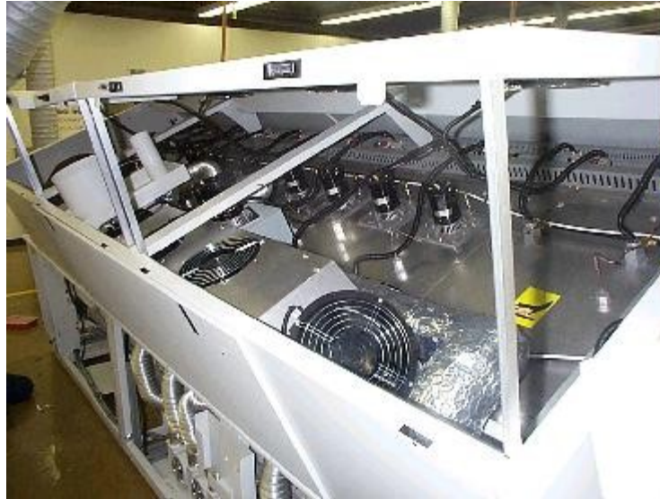
Flux Separation Box Showing Cooling Fans Photo 1
